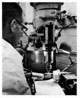
CERAMIC MATERIAL is positioned on a metal holding plate (to relieve strain on soft material) as Charles Ladig (7142-4) operates this mill. Flexible hose connected to a commercial vacuum cleaner keeps machined part clean and prevents inhalation of ceramic dust.
